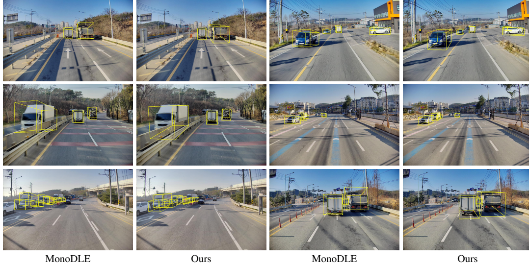
Figure 4. Qualitative results of the baseline model (MonoDLE [11]) and our method on real-world datasets. Training datasets are captured with a passenger car and test datasets are captured with a truck. We visualize the regressed 3D bounding box from MonoDLE and ours.
