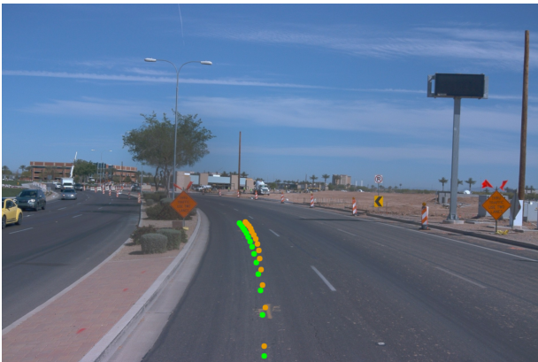
Figure 5. An example of the ground-truth future waypoints (green) and waypoints predicted by our model (orange). The predictions are for 1.6s into the future after the last frame in the input sequence.
