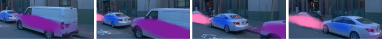
Figure 3. Our model is able to track many vehicles and pedestrians in held-out validation runs from the real-world Waymo Open dataset. We use Hungarian matching to determine best-fit predicted masks for each ground-truth object as described in section 4.2. In this figure, the alpha-value of the colored mask pixels is determined by the weight of the mask at each pixel.
