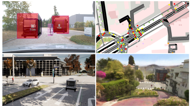
Figure 1. Examples of our proposed simulation levels. Top-left to bottom-right: AR-enhanced (level 1), SUMO (level 2), CARLA (level 3), Block-NeRF (level 4) [59].
